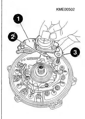
DISMANTLING AND CHECKING ALTERNATOR Dismantling regulator NOTE: This work need not be performed if regulator is replaced. Carefully remove residual adhesive (arrow) at regulator and clean regulator with compressed air (max. 4 bar). ATTENTION: Take care not to damage regulator.
